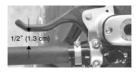
distance indicates low brake fluid level or air in the hydraulic system. Refer to the brake bleeding information on page 80.
